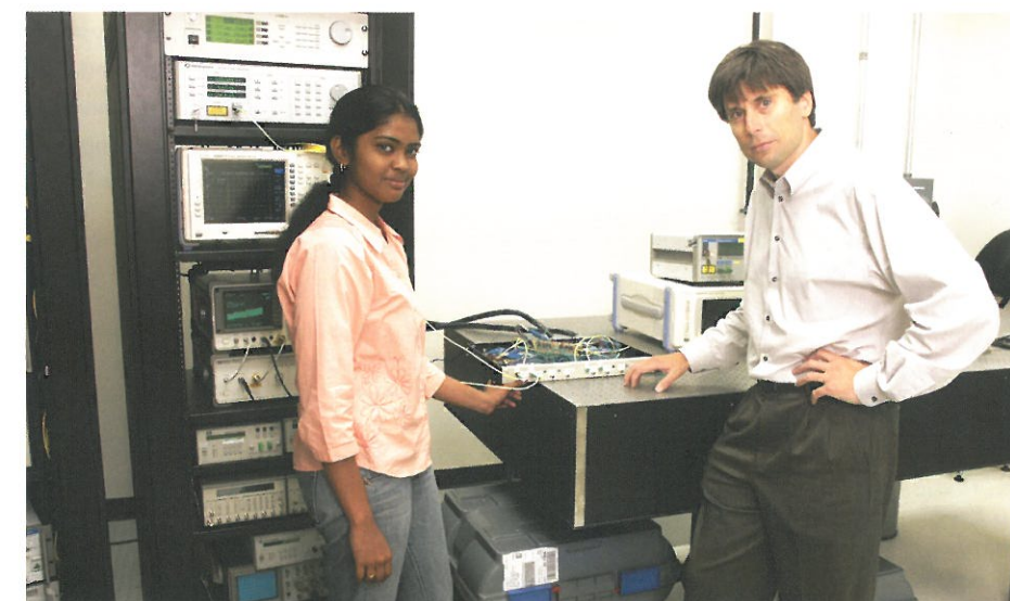
Graduate student Sravanthi Thotakura and Dr. Michael Vasilyev prepare to test an optical amplifier prototype for their 10 Gb/s recirculating-loop testbed. The testbed is used to study the operation and cascability of the novel devices performing nonlinear-optical signal processing of high-speed signals carried by multiple wavelengths.
